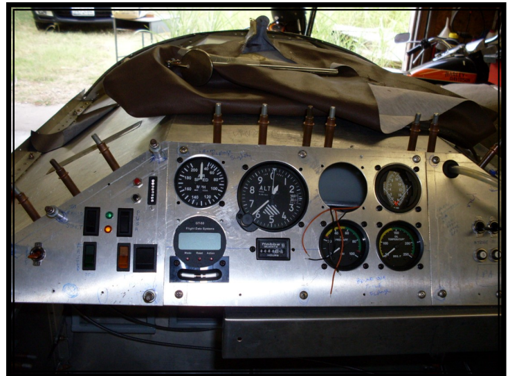
Non Electronic 50 cent fuel gauge. A thin stripe of colored vinyl electrical tape on back side from observer makes the liquid level in the column glow with color.
