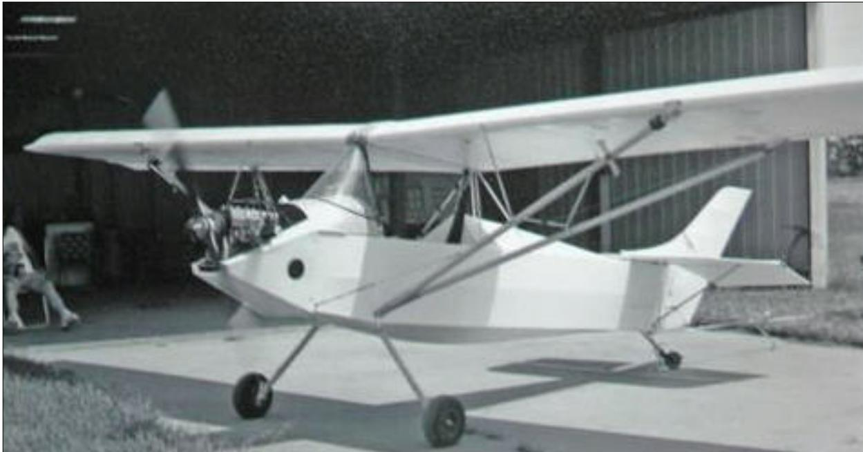
Raceair "Skylite", 1 seat cubalike (Jan 05 Kitplanes) Pro welded 4130 fuselage, alum spars/ ribs, all Stitts covered & paint. 14hrs on 35hp 2Si, Ivo prop. Well built, always hangared @ Caddo Mills, 45mi NE Dallas. Plans, jigs, const. photos. \$7200.
