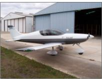
incredible. This little plane weighs less than 600 lbs. empty with a max gross about 1200lbs.
